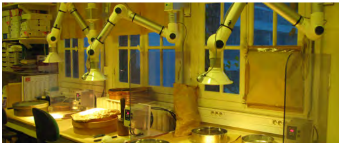
Work bench for seed cleaning, equipped with extractor hoods and cleaning tools (sieves, strainers, pestle and mortar etc.).
